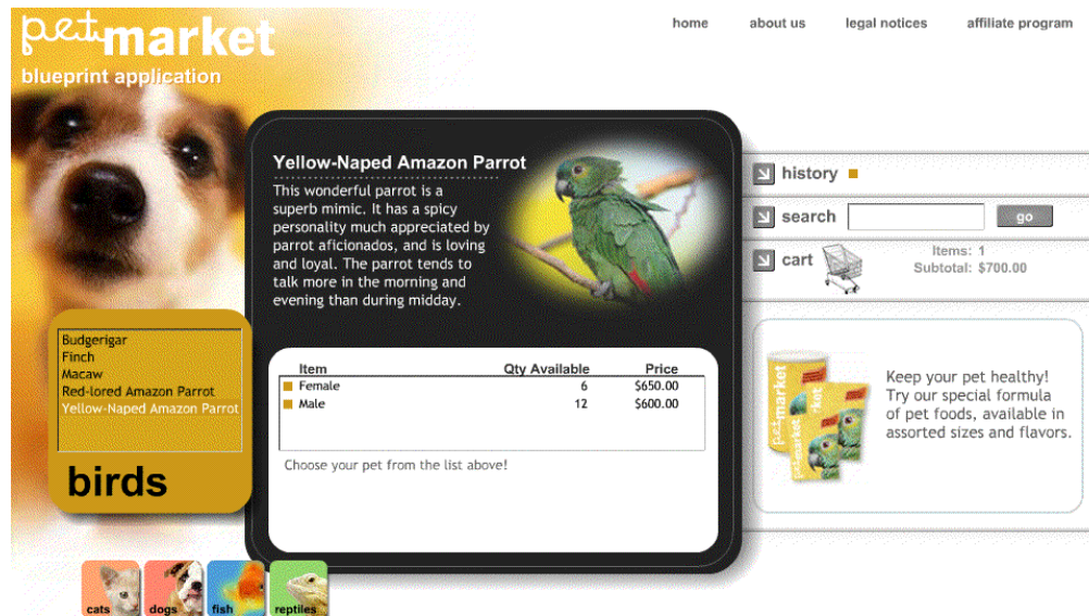
Figure 5, Step 3: When the user selects a bird, the other species’ tabs move down the screen to an auxiliary position making room to display the specific product. The user is now learning about a parrot.
